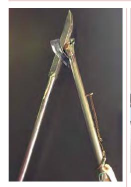
This is a "Detroit" Door Opener which combines an ordinary bar with a hinged, footed, extendable supporting leg. It is used by fire fighters to gain access to locked reinforced doors.
