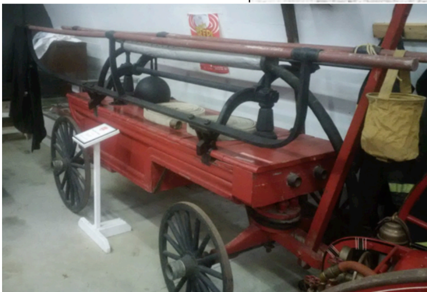
Above: Side stroke “piano-box” engine, CFFM collection on loan from the town of Orillia.
