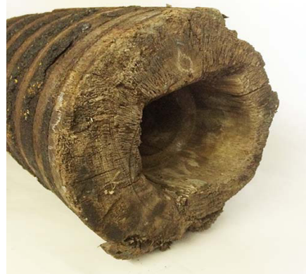
Above: A section of wooden water main believed to be from Quebec City. It would have been bound with metal bands at regular intervals.
